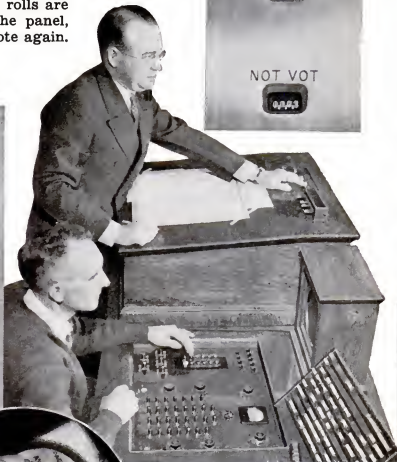
The chief clerk of the Wisconsin State Assembly opens the roll for a record vote, while the voting-machine operator beside him mans the controls. In addition to saving time, the apparatus avoids danger of errors
